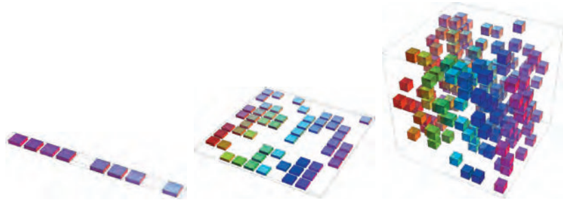
Figure 5.9: As the number of relevant dimensions of the data increases (from left to right), the number of configurations of interest may grow exponentially. ( Left ) In this one-dimensional example, we have one variable for which we only care to distinguish 10 regions of interest. With enough examples falling within each of these regions (each region corresponds to a cell in the illustration), learning algorithms can easily generalize correctly. A straightforward way to generalize is to estimate the value of the target function within each region (and possibly interpolate between neighboring regions). ( Center ) With two dimensions, it is more difficult to distinguish 10 different values of each variable. We need to keep track of up to 10 \times 10 = 100 regions, and we need at least that many examples to cover all those regions. ( Right ) With three dimensions, this grows to 10^3 = 1,000 regions and at least that many examples. For d dimensions and v values to be distinguished along each axis, we seem to need O(v^d) regions and examples. This is an instance of the curse of dimensionality. Figure graciously provided by Nicolas Chapados.
